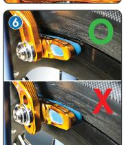
Fine tune the brake pad position in the bracking track surface, leaving a gap of 1 or 2 mm. Tighten the bolts with a 4 mm hex wrench.
