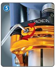
If the caliper is not centered, use a 2,5 mm hex wrench to fine tuning the caliper position turning the fine adjustment screw.
